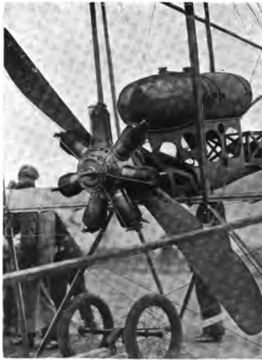
THE GNOME ENGINE PROPELLER AND FUEL TANK OF PAULHAN'S FARMAN BIPLANE
